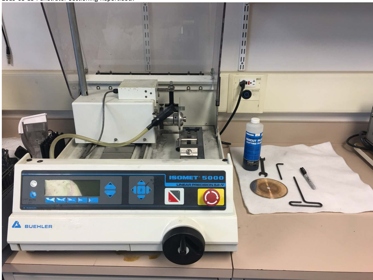
Fig 9. (Sample 3). Isomet 5000 automated sectioning saw setup#
