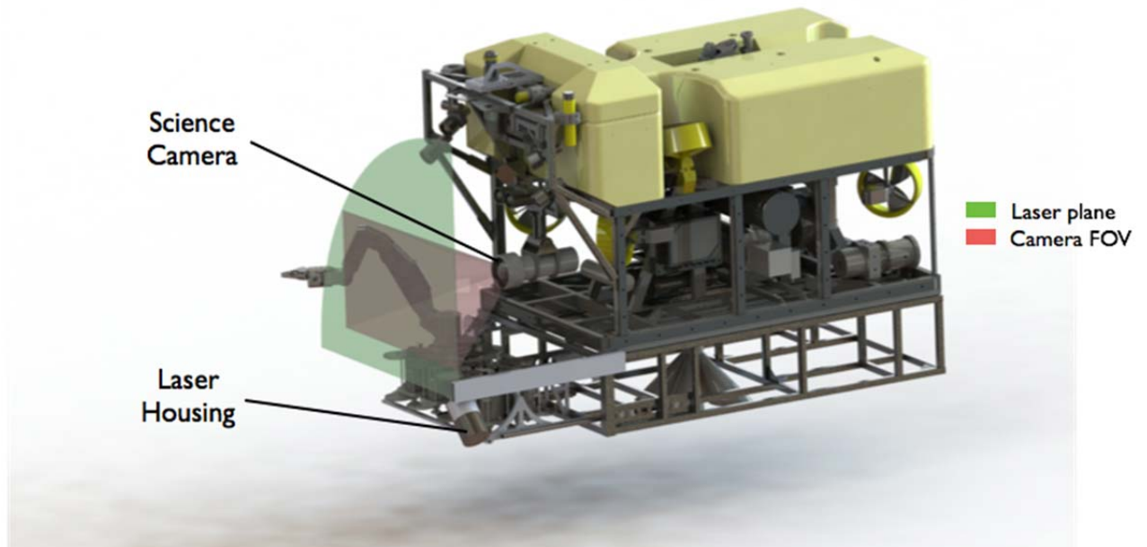
Figure 4. Preliminary design of DeepPIV deployed on ROV Doc Ricketts. The laser sheet is 1 mm in front of the science camera and illuminates approximately 1.5 m 2 field of view using a 90 deg spread angle optic.
