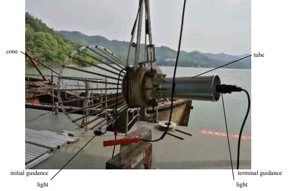
Fig. 2 structure of the dock
