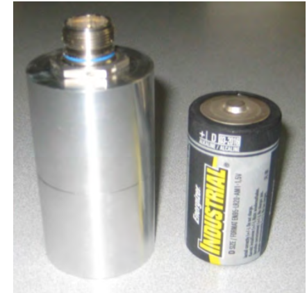
Hermetically sealed 2We TAPS battery next to D-cell
