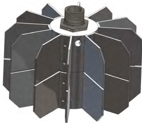
TAPS Battery with Cooling Fins
