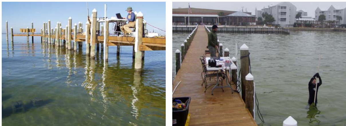
Figure 26. Photographs of the dock site from which data collection was facilitated. The seafloor consisted of fine sands and silt and had very little variation in relief. Water depths ranged from 1 to 3 meters over the site. Semi-diurnal tides of 14-27 cm did not influence water depths significantly.
