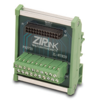
ZL-RTB20 20-pin feed-through connector module
