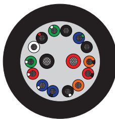
Type: P7TP22/2C18# 7 twisted pairs, 22 AWG 2 conductors, 18 AWG Nom. cable OD: 0.480", 12.20 mm
