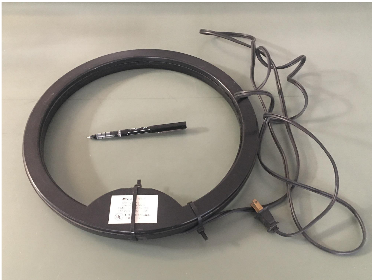
Fig 8. Degaussing coil example
