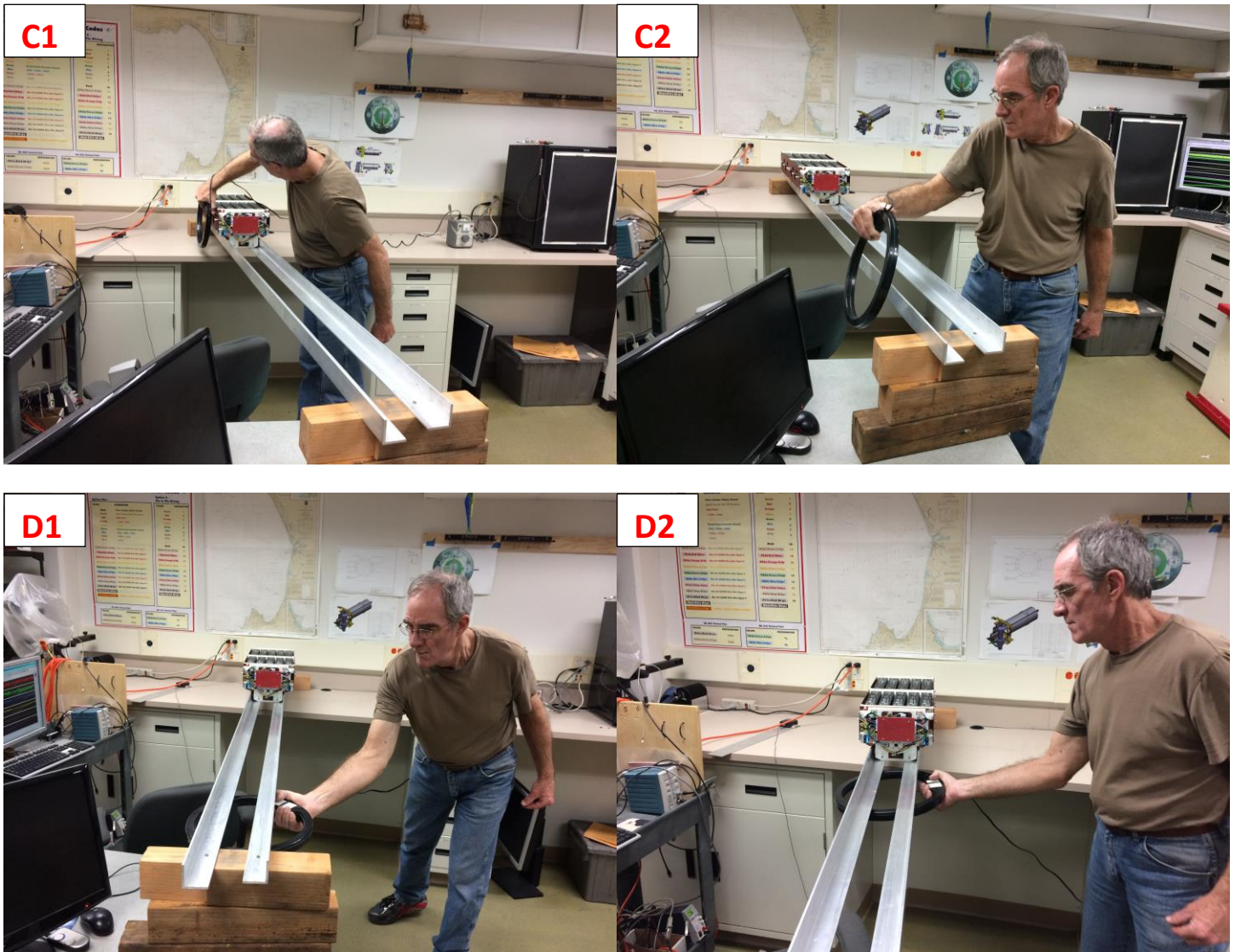
Fig 17. Example of degaussing sequence C1-C2: degaussing Starboard surface D1-D2: degaussing Bottom surface
