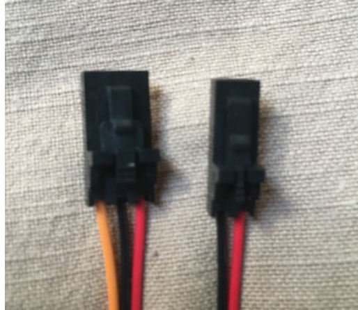
Pump/Valve (C-Grid 2/3 pin)]
