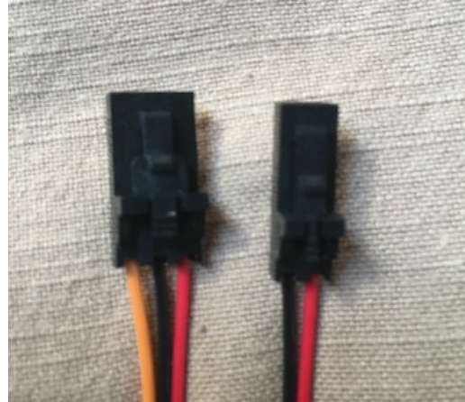
Pump/Valve (C-Grid 2/3 pin)]
