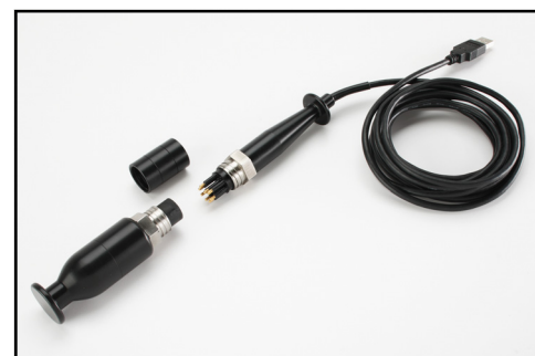
LISST-HOLO memory module and USB offload cable (1 set included)
