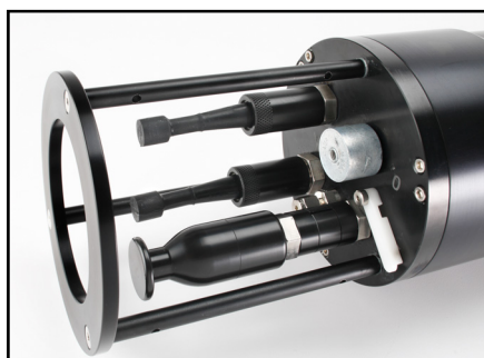
Connector endcap with external memory module for easy offloading of holograms
