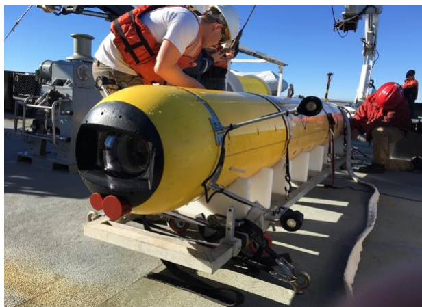
Figure 1. Pre-dive operations on the assembled i2MAP+A vehicle, the forward transducers are the red cylinders below the camera dome.
