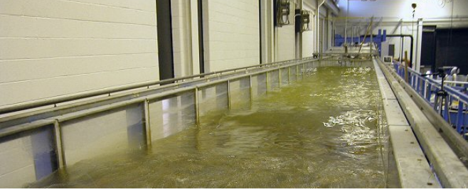
Figure 2. Our short-range high-frequency acoustic communication testbed: A 1.22m \times 1.83m \times 49m flume.
