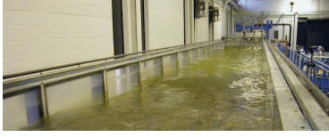
Fig. 1. Our short-range high-frequency acoustic communication testbed: a 1.22\text{m} \times 1.83\text{m} \times 49\text{m} flume.
