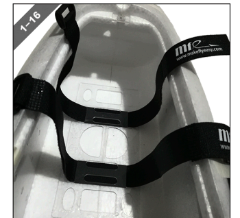
图1-15/16 先固定魔术扎带，在机身电池板部分涂泡沫胶粘合。 FIGS 1-17/18 Fixed the magic tie straps before bonding the fuselage battery panel with foam glue.
