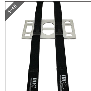
图1-15/16 先固定魔术扎带，在机身电池板部分涂泡沫胶粘合。 FIGS 1-17/18 Fixed the magic tie straps before bonding the fuselage battery panel with foam glue.
