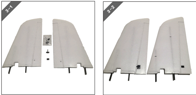
图3-1/2 尾翼舵角、舵角压片涂泡沫胶安装在尾翼舵面，并用M2*8断尾螺丝固定。 FIGS 3-1/2 The helm angle and helm angle presser should be coated with foam glue and installing them on the helm surface of empennage, fixed them with M2*8 tail screw.
