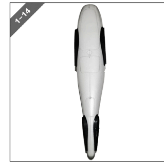
图1-13/14 合模前，请务必检查机身内的配件都已安装。在机身剖面部分涂上泡沫胶，合模。注意：合模时要对齐、压紧，机翼和尾翼的机身塑料件也用泡沫胶粘合。 FIGS 1-13/14 Ensure all parts of the fuselage has been installed before die assembly. Coating the cross-section of fuselage with foam glue and then conduct the die assembly. Attentions: ensure the die were consistent with each other and toughly pressed while conducting the die assembly, the plastic parts of the wing and empennage should be bonded with foam glue too.
