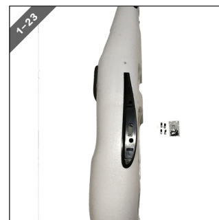
图1-23/24 将锁钩安装在机翼连接件机身部分，并用M2*8断尾螺丝固定。 FIGS. 3-23/24 Installing latching hook on the wing connecting parts of fuselage, fixed them with M2*8 tail screw.
