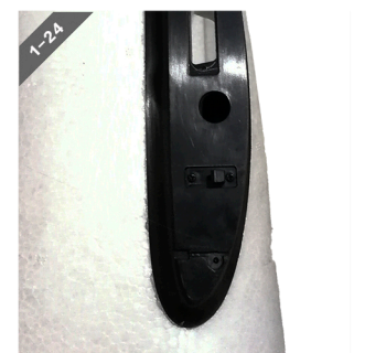
图1-23/24 将锁钩安装在机翼连接件机身部分，并用M2*8断尾螺丝固定。 FIGS. 3-23/24 Installing latching hook on the wing connecting parts of fuselage, fixed them with M2*8 tail screw.
