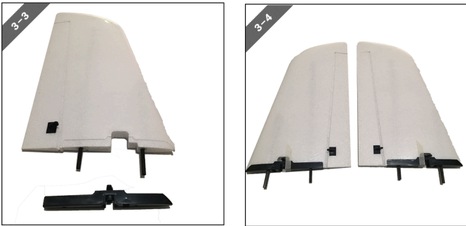
图3-3/4 在尾翼翼根凹处涂泡沫胶，安装尾翼塑料件。 FIGS 3-3/4 Coating foam glue at the recessed position of empennage root. Installing wing plastic parts.
