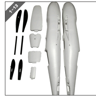
图1-13/14 合模前，请务必检查机身内的配件都已安装。在机身剖面部分涂上泡沫胶，合模。注意：合模时要对齐、压紧，机翼和尾翼的机身塑料件也用泡沫胶粘合。 FIGS 1-13/14 Ensure all parts of the fuselage has been installed before die assembly. Coating the cross-section of fuselage with foam glue and then conduct the die assembly. Attentions: ensure the die were consistent with each other and toughly pressed while conducting the die assembly, the plastic parts of the wing and empennage should be bonded with foam glue too.
