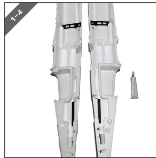
图1-3/4 机身加强板安装在机身中，并用泡沫胶粘合。 FIGS 1-3/4 Installing the fuselage stiffening plate on fuselage and connected them by foam glue.
