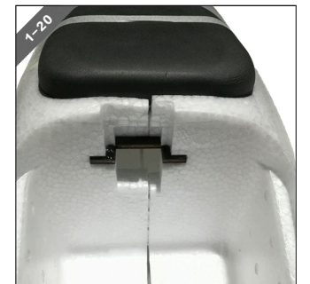
图1-19/20 安装伞舱舵机座，并用泡沫胶粘合。 FIGS 1-19/20 Installing the basement of parachute hatch cover and bonding with foam glue.
