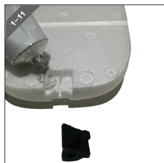
图1-11/12 在电池舱盖、飞控舱盖、图传舱盖凹陷处涂泡沫胶，粘合舱盖锁钉。 FIGS 1-11/12 Coating foam glue at the recessed position of battery cabin, autopilot cabin and image transmission cabin, bonding the hatch cover locking nail.
