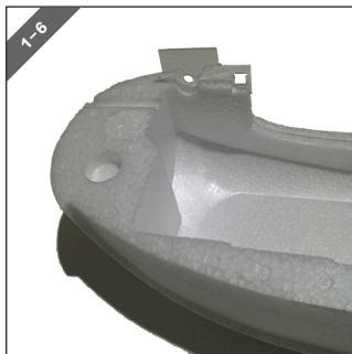
图1-5/6 在电池舱盖和飞控舱盖位置安装舱盖固定板，并用泡沫胶粘合。 FIGS 1-5/6 The cabin cover fixed plate should be installed on the position of battery and autopilot cabin, bonding them with foam glue.
