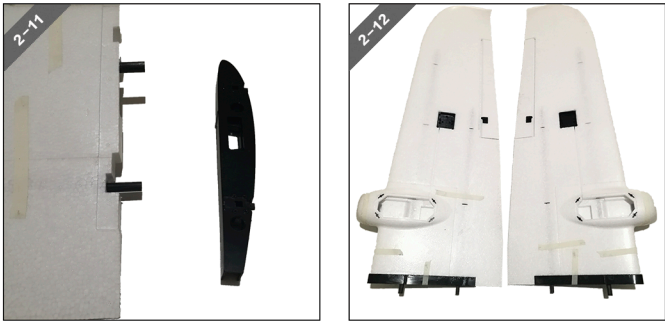
图2-11/12 机翼翼根凹处涂泡沫胶，安装机翼塑料件，用纸胶固定。 FIGS 2-11/12 Coating foam glue at the recessed position of aileron root. Installing wing plastic parts, fixing by paper glue.
