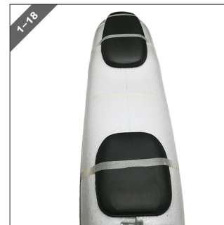
图1-17/18 先将EVA缓冲垫试装在机身底部，并用剪刀剪去EVA边缘多余部分，再用泡沫胶粘合。 FIGS 1-17/18 Trail assembling the EVA cushion on the bottom of fuselage, bonding them with foam glue before cutting the extra parts of EVA cushion edge.
