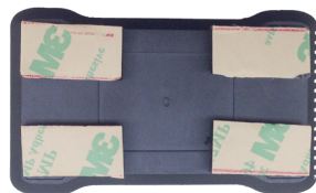
example of foam attached to the bottom of Pixhawk
