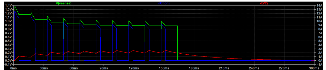
LT spice simulation of 60 Hz, 4ms flashes with flash current, monitor voltage and capacitor ripple current
