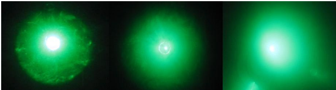
Figure 4-3 Images showing the effects of multiple scattering in water for increased concentrations of Maalox ® (Left to Right)
