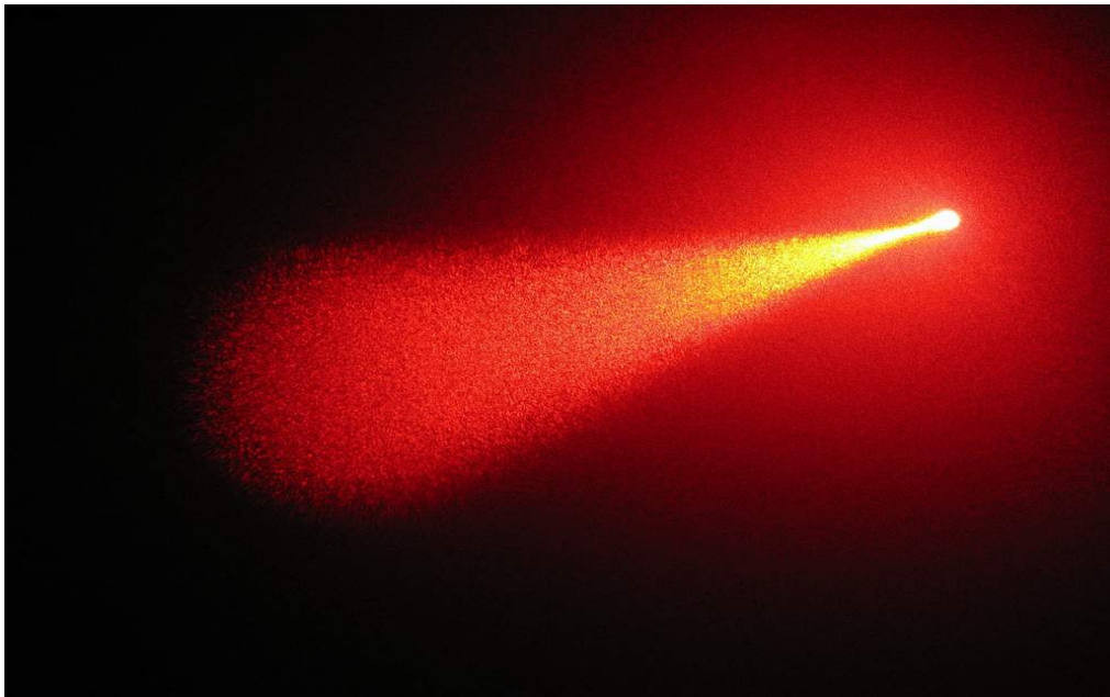
Figure 4-1 Scattering observed in sea water using a Red He-Ne Laser
