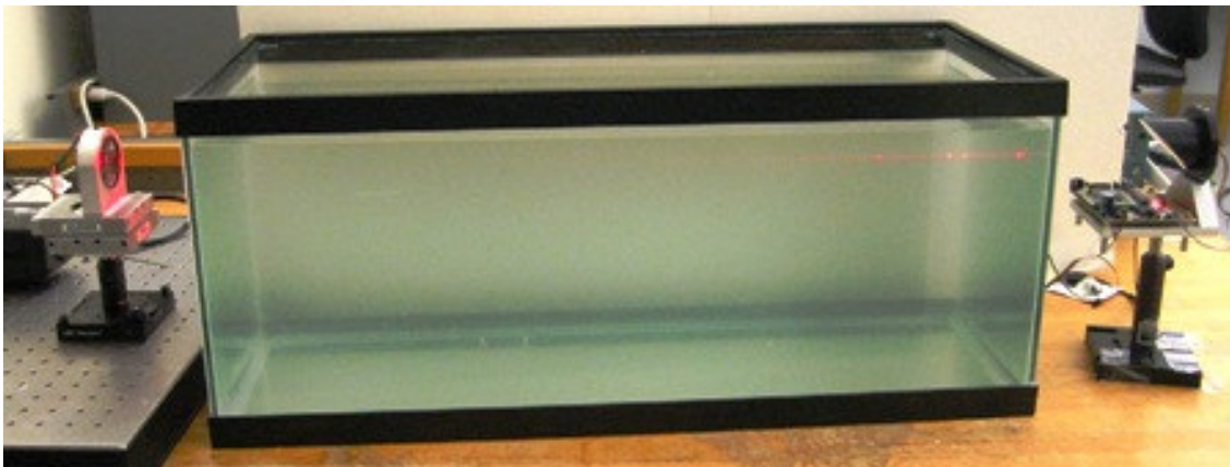
Figure C-1 Underwater experiment tank filled with 5mL of Maalox® liquid (side view)
