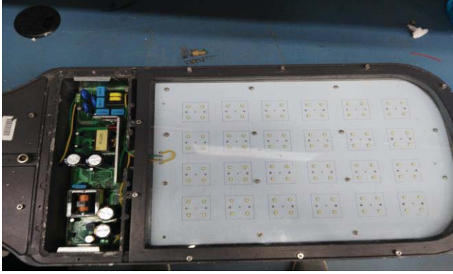
Figure 11. Testing setup with driver,load and fixture
