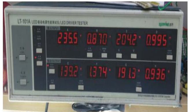
Figure 9. Electrical test parameters from power analyzer
