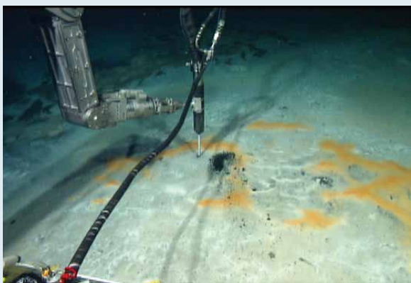
The ROV inserts a laser Raman spectrometer probe into the seafloor to take in situ measurements of this methane-rich area covered in bacterial mats.
