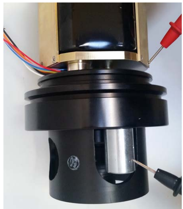
Figure 9-3 Checking the Sacrificial Anode of an ATM-964 or ATM-965 Acoustic Telemetry Modem
