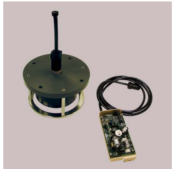
Figure 1-15 The ATM-903 Modem Board Set (Shown with Omnidirectional LF Transducer)
