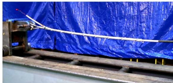
PMI CABLE-GRIP™ Termination shown applied on cable under tension.
