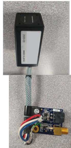
PMT: 50 x 22 x 22 mm PCB: 37 x 25 x 14 mm
