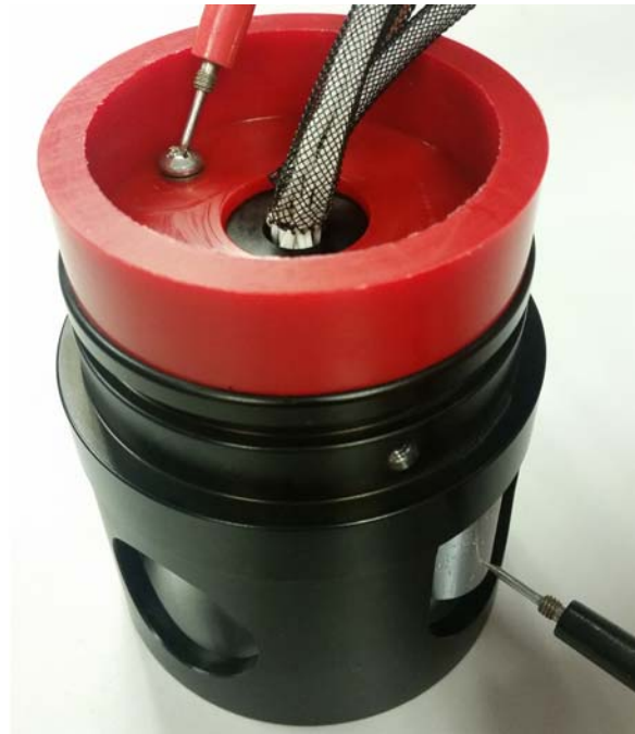
Figure 9-1 Checking the Sacrificial Anode of an ATM-924 or ATM-925 Acoustic Telemetry Modem
