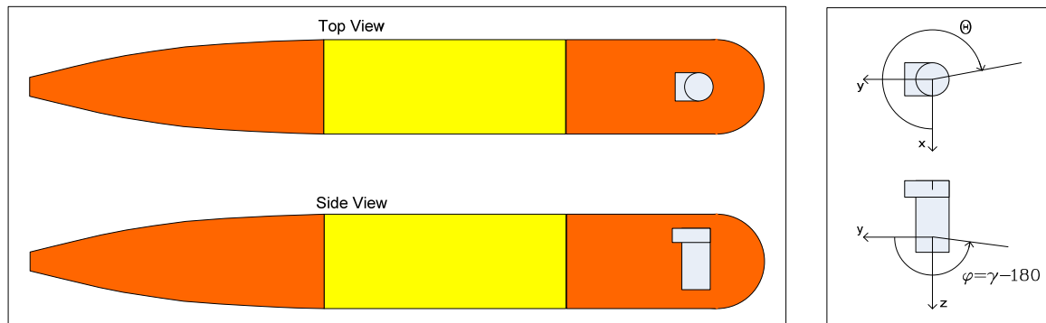
Figure 1: Current arrangement of USBL in vehicle and the sensors coordinate system.
