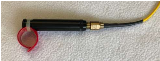
Tether penetrator (covered by its black plastic protective cap)
