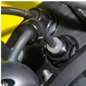
Before cap is screwed back on Cap should be finger tight
