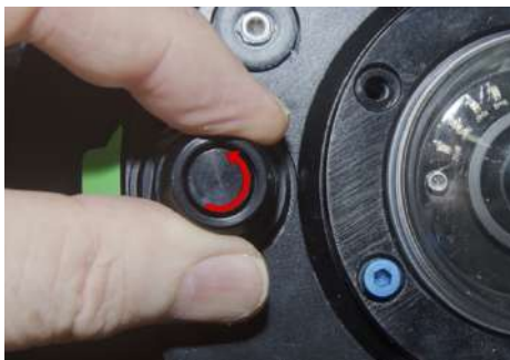
Unscrewing cap from vacuum port
