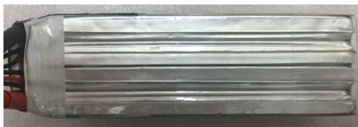
Side view showing four cells inside battery
