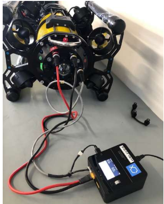
Boxfish ROV charge cables and charger connected in preparation for charging
