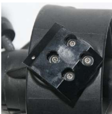
Thruster mounting plate attached to cowling
