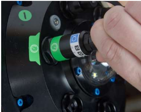
Holding the vacuum hose in place while pressurising the ROV
