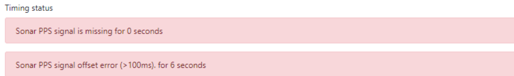
Figure 27. Errors associated with PPS noise
