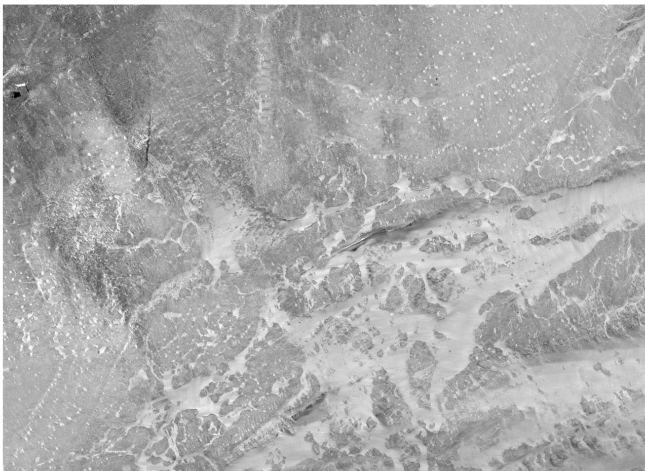
NORBIT Snippets-Sidescan Backscatter 50cm resolution Mosaic data from 30m water depth
