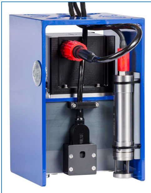
Figure 123: Aft detail of the IMU cable connection
