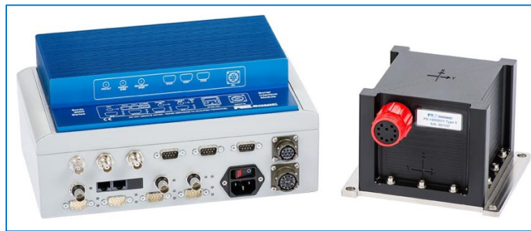
Figure 118: R2Sonic I2NS Main Components (not including antennas and cables)
