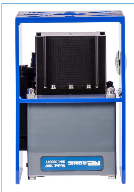
Figure 121: IMU mounted within the Sonic 2022 mounting frame
