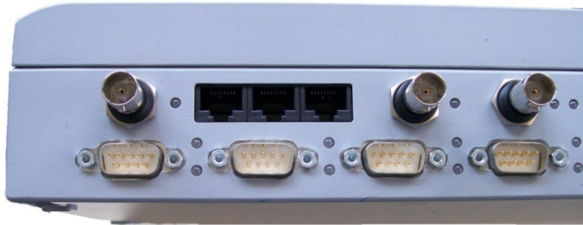
Figure 14: SIM Interfacing Physical Connections
