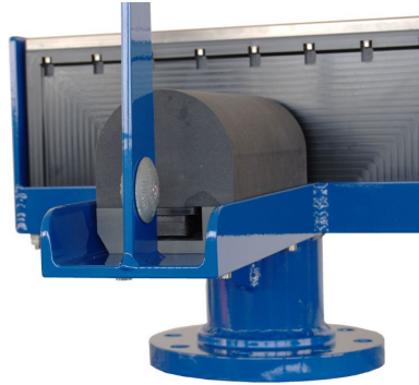
Figure 30: View of the mounted Projector; NB. The connector is facing protective fin
