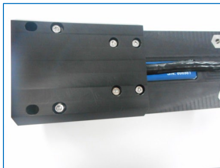
Figure 23: Projector cable clamp in place
