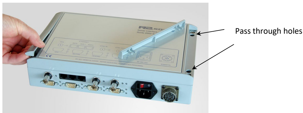
Figure 36: Removal of trim to expose securing holes
