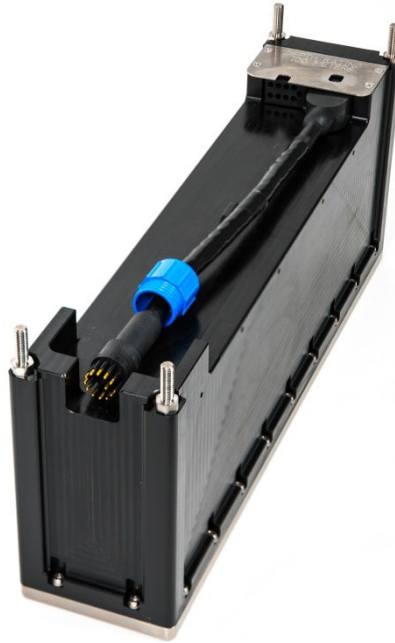
Figure 13: New cable penetrator with a locking ring
