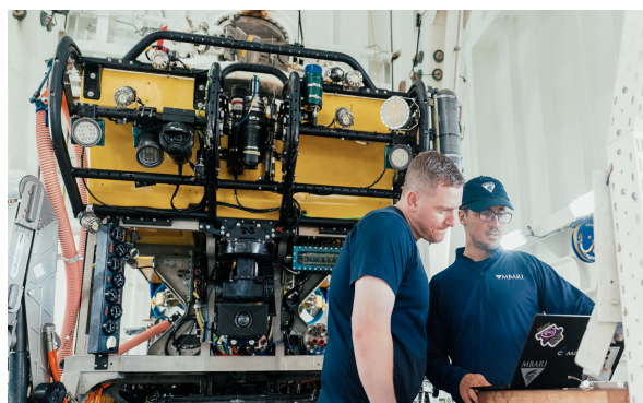
Figure: Compact sled adapted from CoMPAS MiniROV Mapping sled mounted on ROV SuBastian (left) thanks to a collaborative effort with SOI ROV pilots (right).
