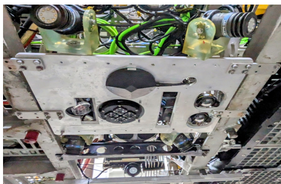
Figure: Compact sled adapted from CoMPAS MiniROV Mapping sled mounted on ROV SuBastian (left) thanks to a collaborative effort with SOI ROV pilots (right).
