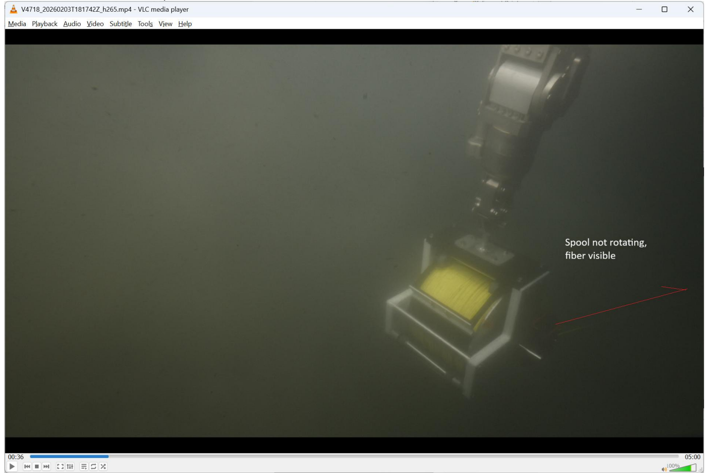
Fig. 29. T-minus 01:04 to Second Strain Event. Spool not rotating, fiber visible more straight from the spool
