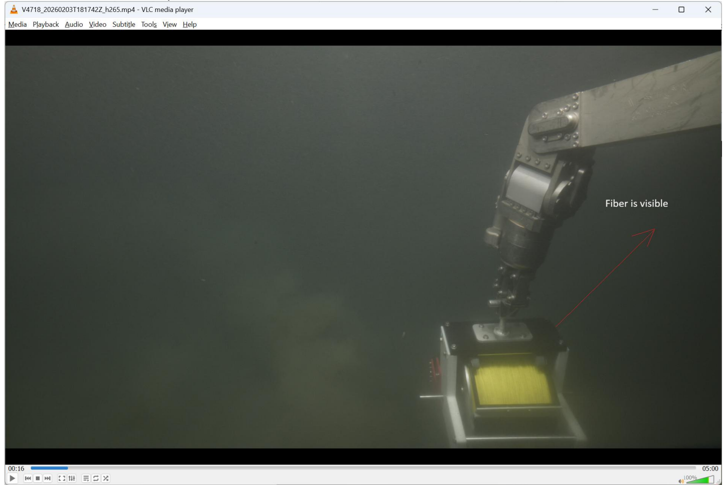
Fig 22. T-plus 00:05 from First Strain Event; T-minus 01:24 to Second Strain Event. Fiber is visible, spool rotating
