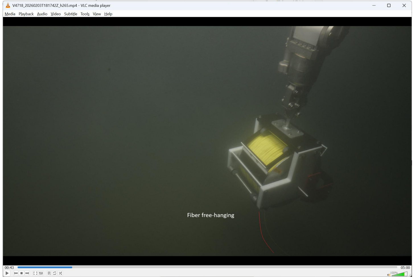
Fig. 31. T-minus 00:57 to Second Strain Event. Fiber is visible, it is free-hanging down from the spool.
