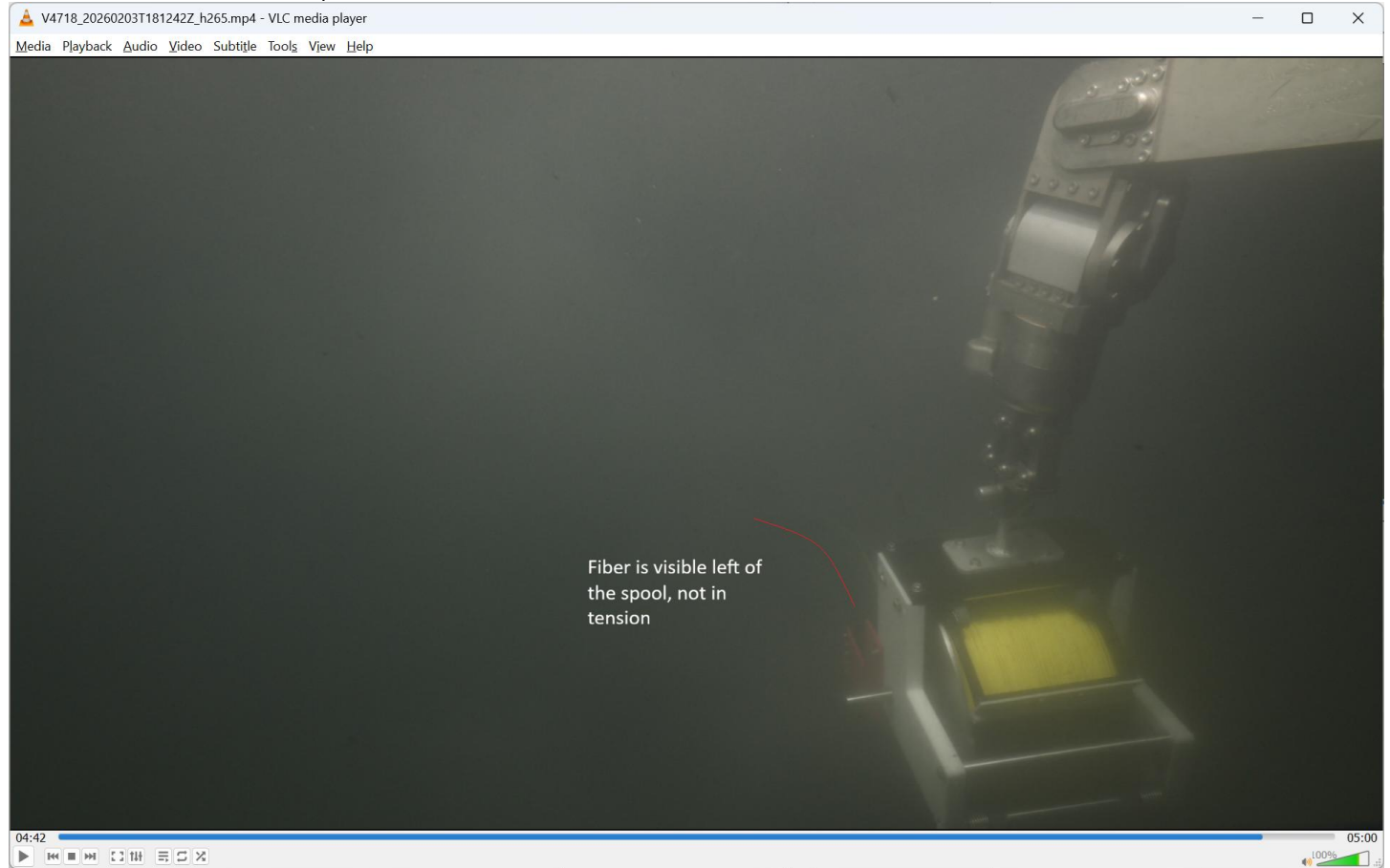
Fig 14. T-minus 00:29 to First Strain Event. Fiber is visible left of the spool, not in tension.
