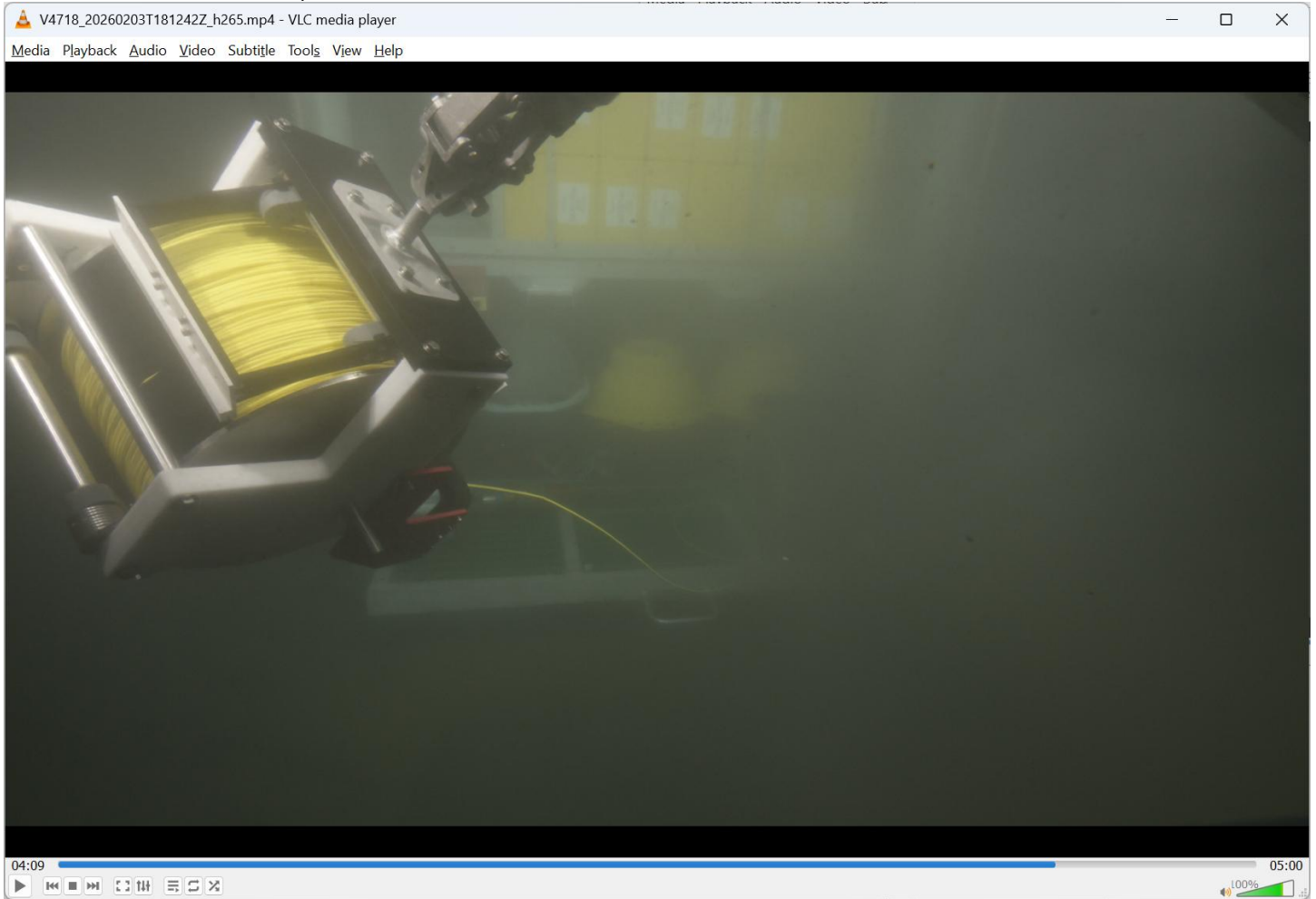
Fig 12. T-minus 01:02 to First Strain Event. Fiber is freed from under the tub, "Alana said; You got it!", distance ~ 3 m, 2 fiber loops visible.
