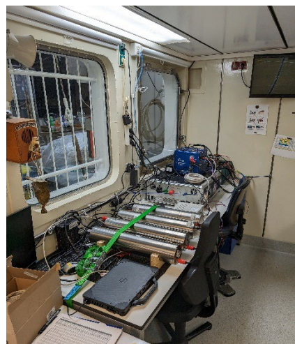
Fig. 5.4 Lap setup of the SWAN system in the dry lab. The four metal tubes are the receiver logger units, which were fitted into a POM housing and connected to the receiver dipoles for acquisition.
