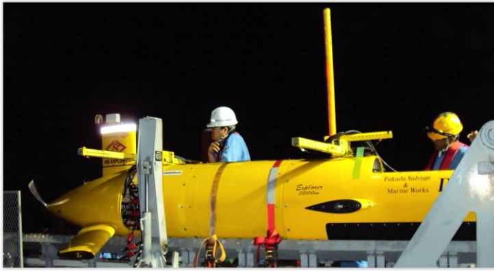
Fig. 4: AUV CSEM survey, Sea of Japan Nov 2016. Left, AUV with electric dipole mounts on AUV, including a vertical pair of electrodes. Right, Scripps DUESI seafloor transmitter being deployed.
