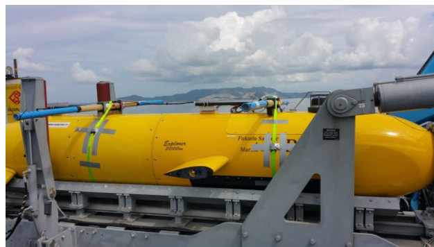
Fig. 1: The first (2015) test set up with a pair of electrodes mounted on top of Fukada's Deep1 AUV.
