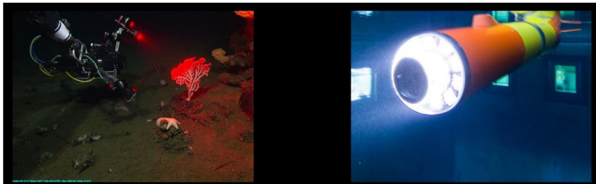
Figure 1: (left) The ROV-deployed plenoptic imaging system EyeRIS imaging a deep sea coral (right) the multi-camera 3D imaging system AyeRIS integrated into MBARI's Long-Range AUV in the test tank
