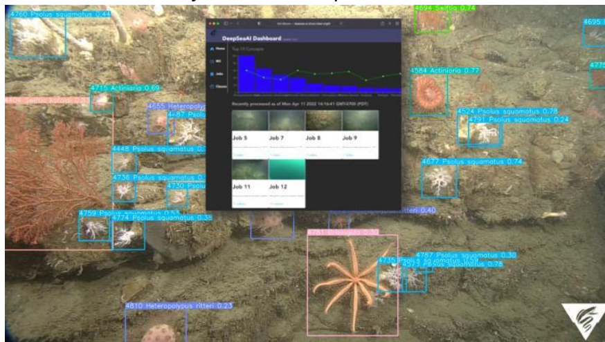
Figure 1: Top-level view of the web dashboard and example detections from our YOLOv5 detection and DeepSort tracking pipeline
