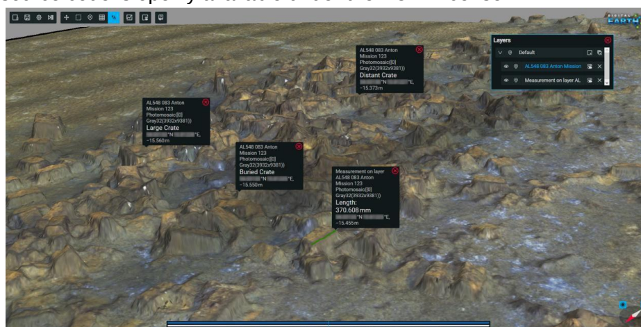
Figure 1: Photogrammetric reconstruction of subsea munitions in the Digital Earth Viewer with annotations and measurements
