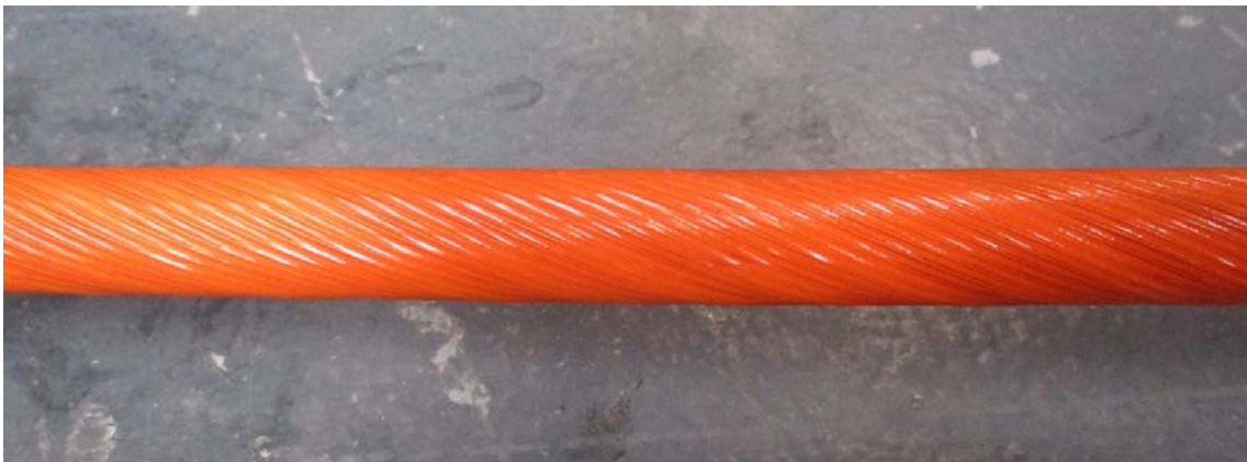
Figure 9.16: Polyethylene sheath in the region of the “red” tangent point (after cleaning). The left hand side of the sample was straight, right hand, bent (during the test).
