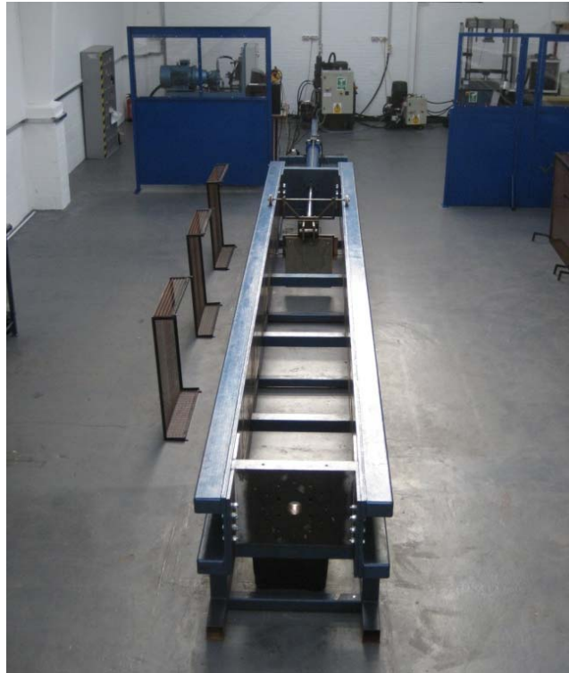
Figure 3.1: 200 kN testing machine at TTI Testing's laboratory in Wallingford, UK.
