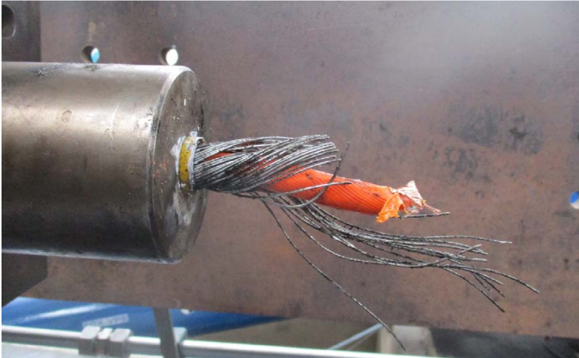
Figure 9.4: Appearance of the cable failure after testing to breaking load (actuator end termination).
