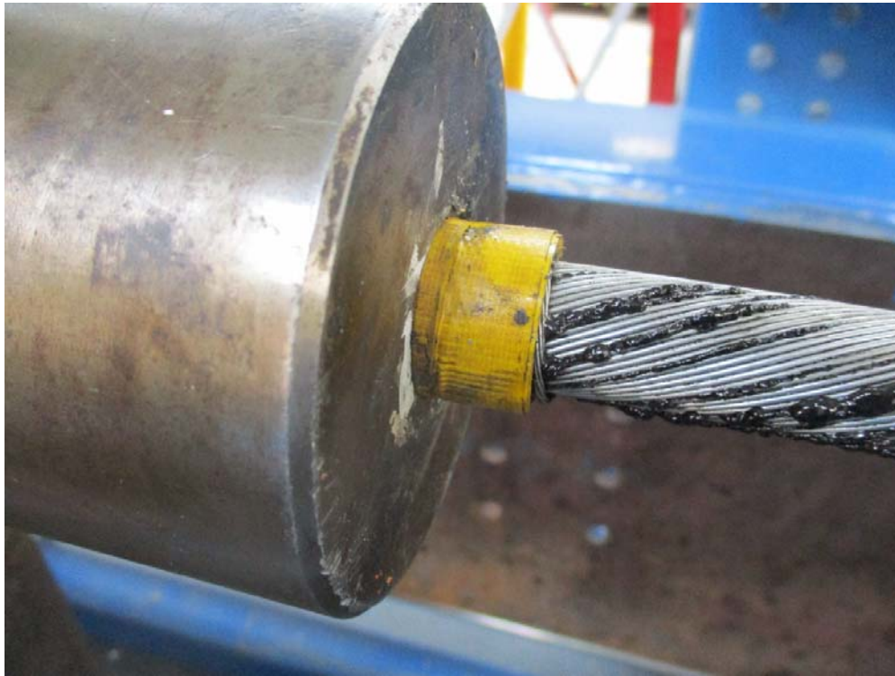
Figure 9.7: Socket draw of approximately 3 – 4 mm noted after 1,000 cycles. Grease has squeezed out from inside the cable (to be expected).
