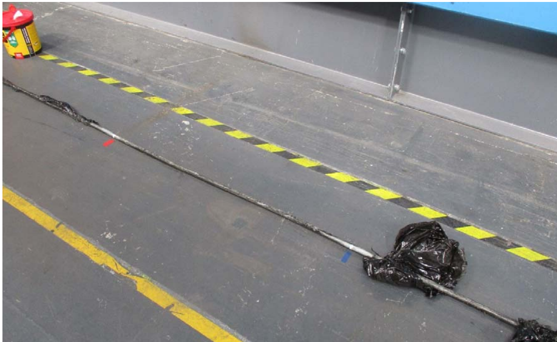
Figure 9.11: Bent T-T test sample laid out for dissection.
