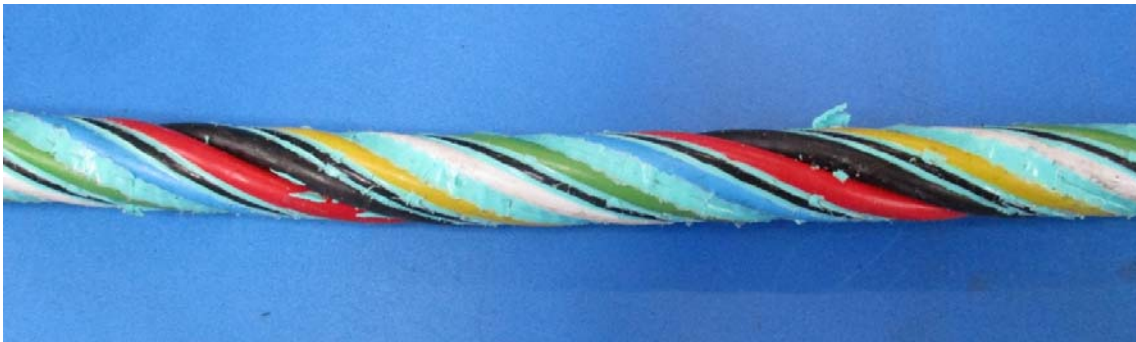
Figure 9.18: Larger power conductors and fibre optic tube, drain wires and silicone rubber compound.
