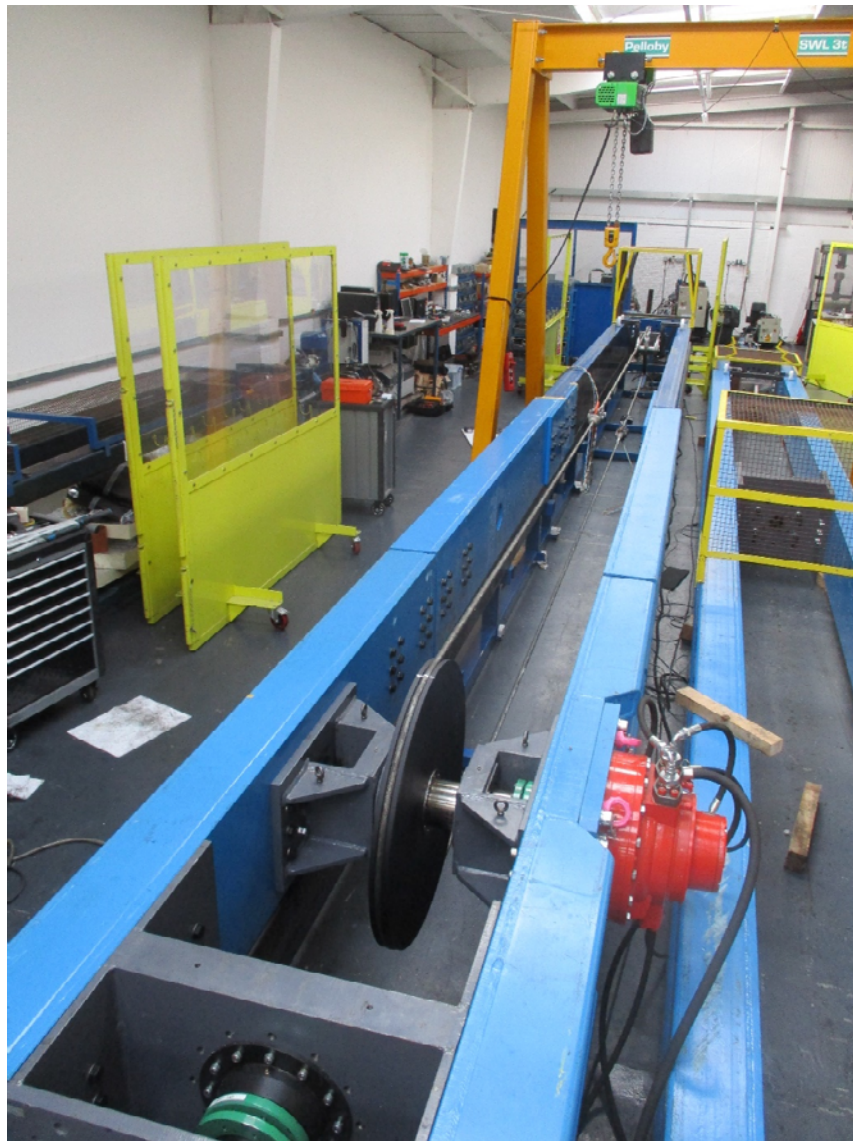
Figure 9.21: 200 kN machine set up to run the CBoS test.
