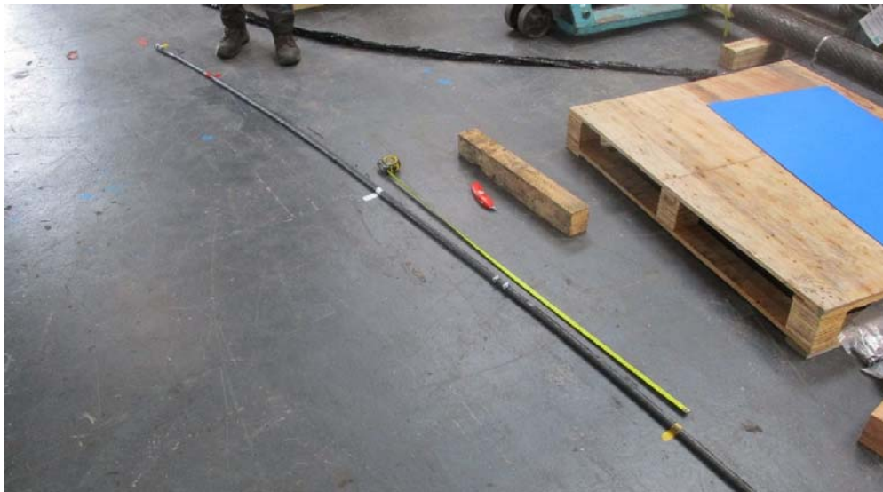
Figure 9.26: CBoS sample laid out for inspection. The red tape marks the top always straight-SBZ interface. The top SBZ is between red and white tape, and DBZ between white and yellow. The second SBZ is yellow to blue (not shown).
