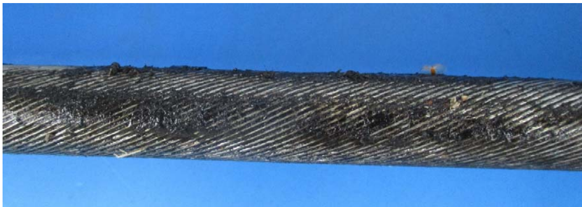
Figure 9.12: Section of sample which has been bent over the sheave – the heavier lubricant deposit on the section which had faced away from the groove.
