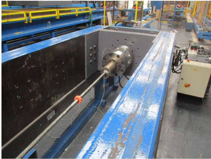
Figure 9.2: View on rotation crosshead showing torsion load cell and elongation clamp.
