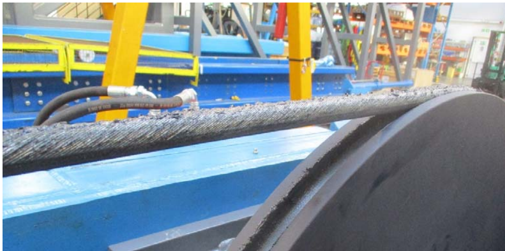
Figure 9.28: CBoS sample in test machine showing the distribution of grease around the cable on a section which has operated over the sheave.
