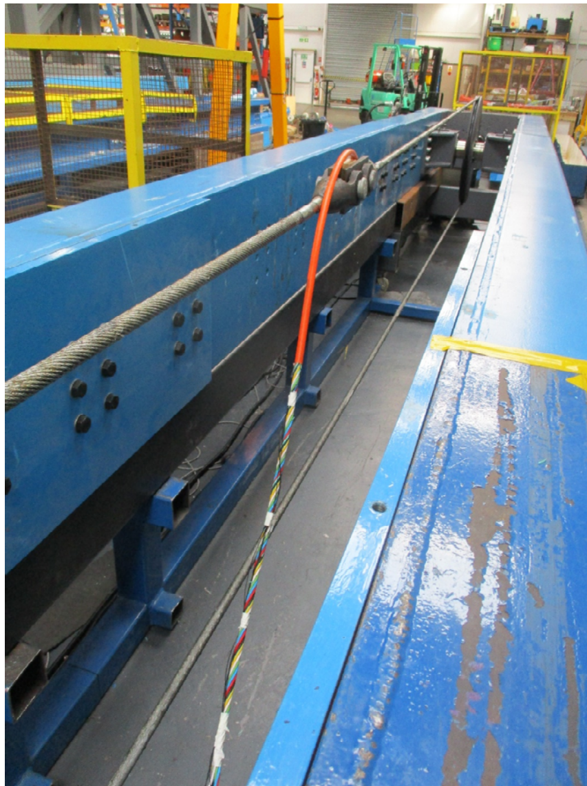
Figure 9.22: View on CBoS test looking towards the test sheave (dummy rope top left), a long pigtail was employed to allow for the movement during the bend cycling.
