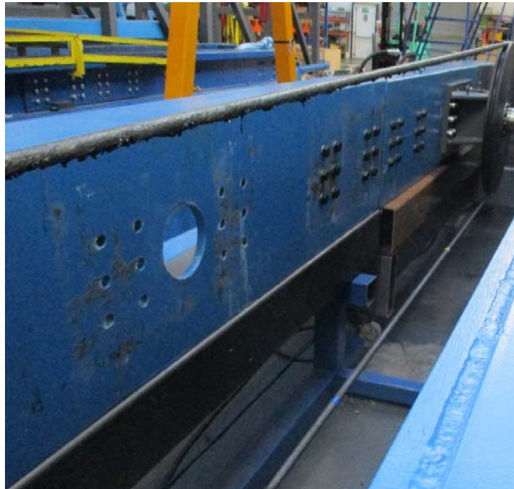
Figure 9.27: CBoS sample in test machine during marking of the bending zones. At the top is a section of always straight cable, and the collection of grease along the bottom side may clearly be seen (the blue – yellow SBZ can be seen at the bottom).
