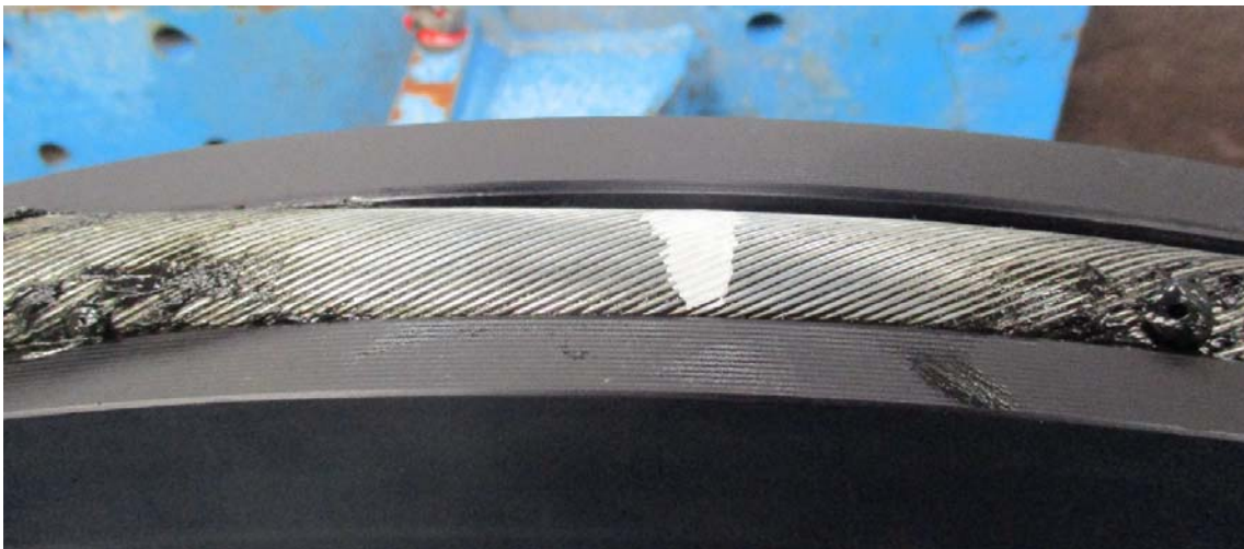
Figure 9.10: Detailed view on cleaned tangent point area on the sample on completion of 7,500 cycles (before removal for inspection) – the condition is very good.
