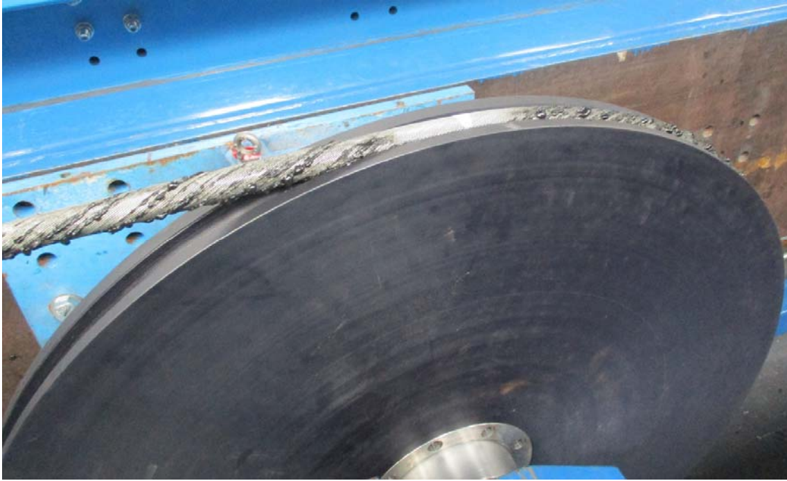
Figure 9.9: Cable on test sheave on completion of 7,500 cycles. Note the tangent point area has been cleaned to aid marking on the sample.
