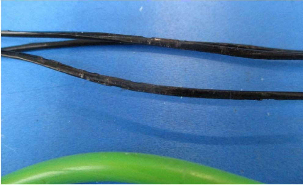
Figure 9.19: Distortion noted on the coating of the drain wires in the region of the red tangent point.
