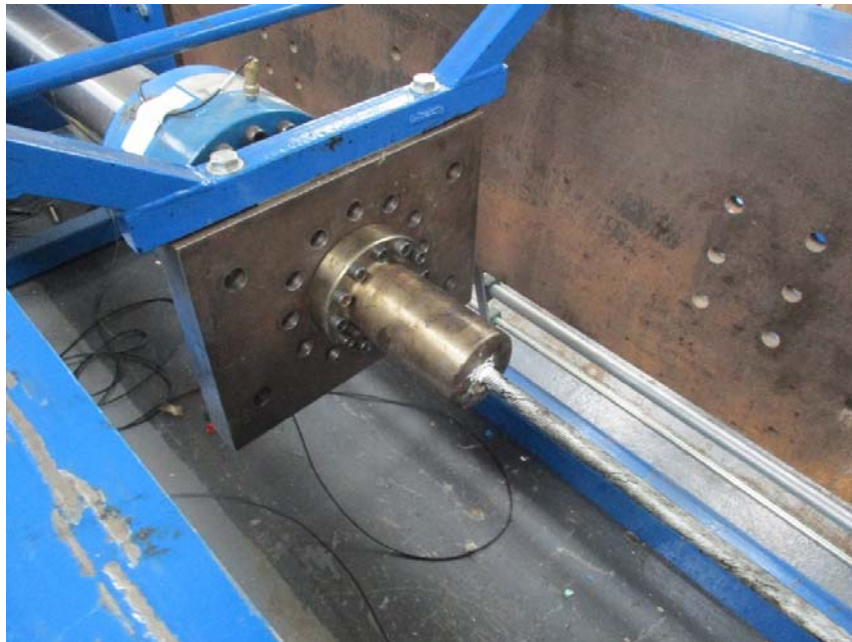
Figure 2.2: Example showing armoured cable terminated in TTI Testing top-hat end fitting.
