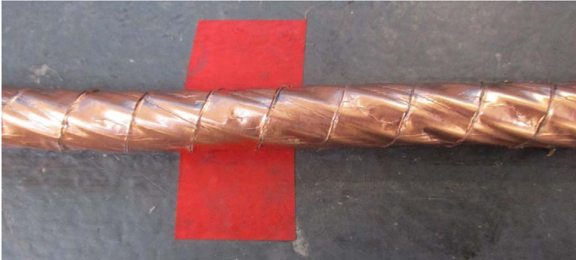
Figure 9.17: Copper/polyester laminate tape wrapping in the region of the “red” tangent point (after cleaning). The left hand side of the sample was straight, right hand, bent (during the test).
