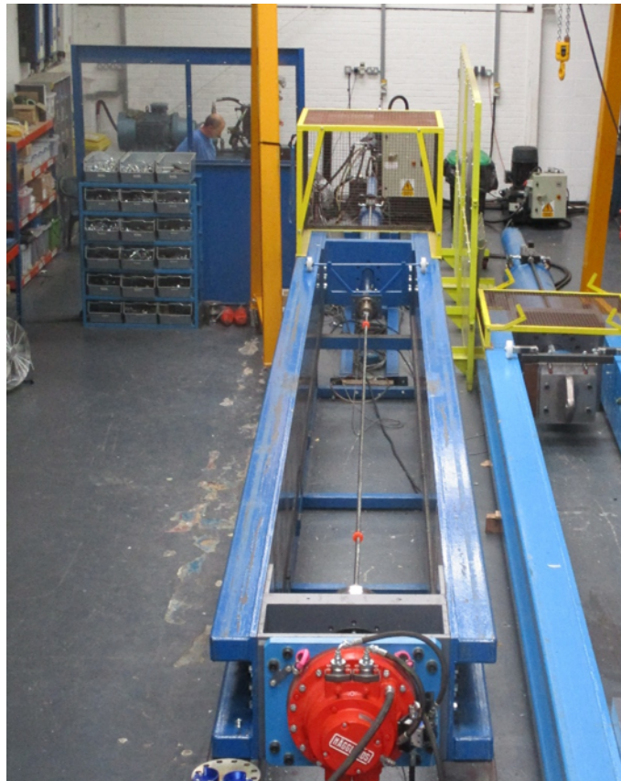
Figure 9.1: Tensile sample mounted in the 200 kN machine for the elongation and rotation test.
