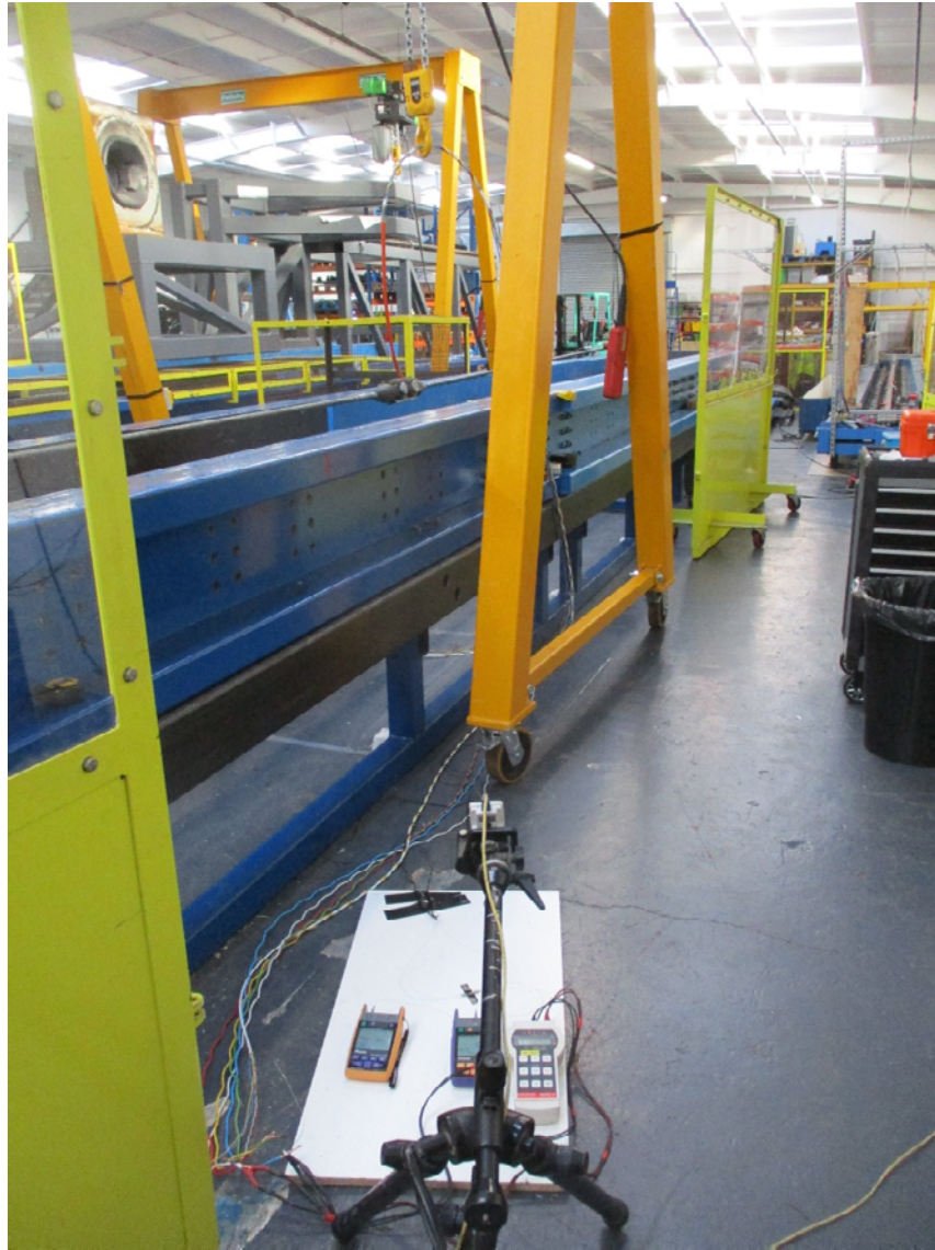
Figure 9.23: View on CBoS test looking towards the test sheave with the long (top) pigtail looped through the hook of the gantry crane in order to prevent it catching on the sample.
