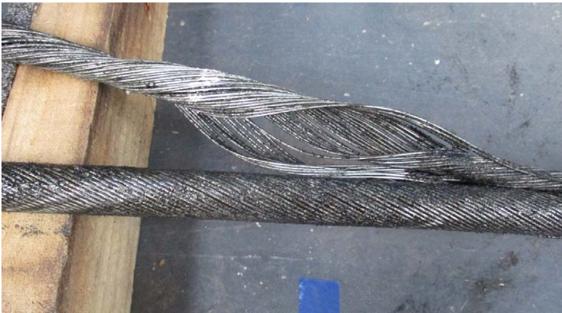
Figure 9.14: Second layer of armour in the region of the "blue" tangent point (note the white paint on the outer layer wires). The second layer lubricant is in good condition and evenly distributed.
