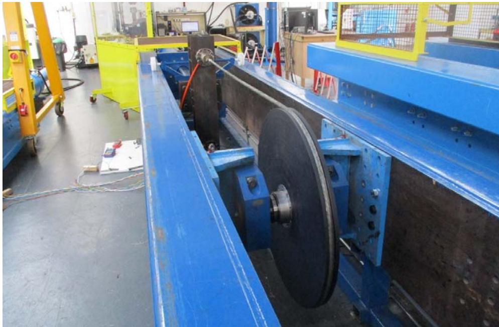
Figure 9.6: Cable set up in 600 kN machine for the start of the Bent T-T test.
