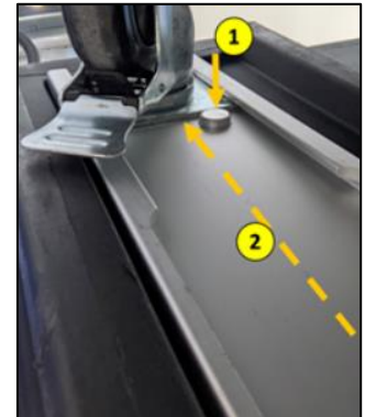
Figure 3 - Installing the wheels
