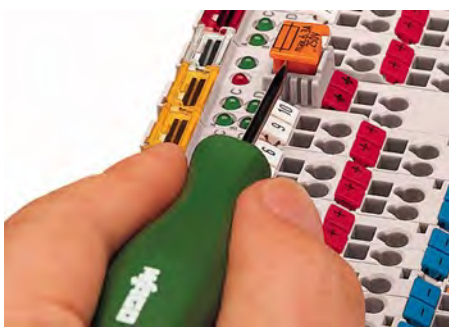
Figure 9: Removing the Fuse Carrier
