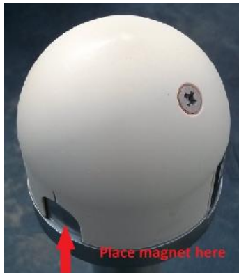
Figure 1: Magnet Placement on Head Assembly
