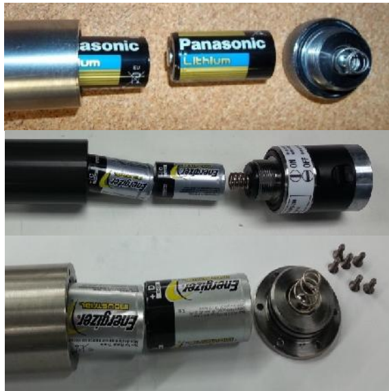
Figure 10: Bottom end caps removed for battery change
