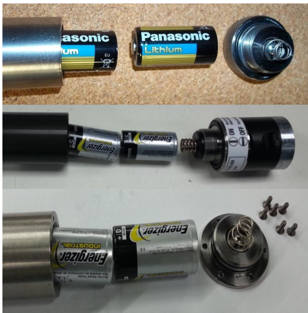
Figure 10: Bottom end caps removed for battery change
