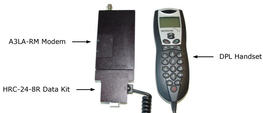
Figure 3. A3LA-RM Connected to a DPL Handset via the HRC-24-8R.
