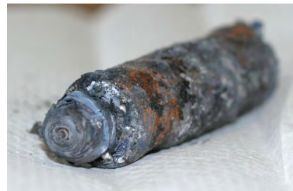
b) Runaway in this cell resulted in aluminum melting (beads can be seen on the end of the jellyroll) and partial ejection of the jellyroll core.
