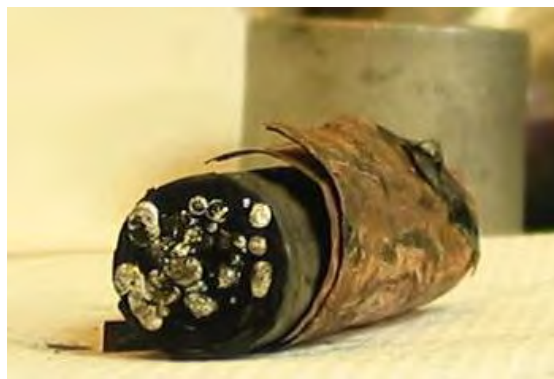
a) This cell ran away after a particle was implanted. Aluminum beads indicate cell temperatures exceeding 660°C.
