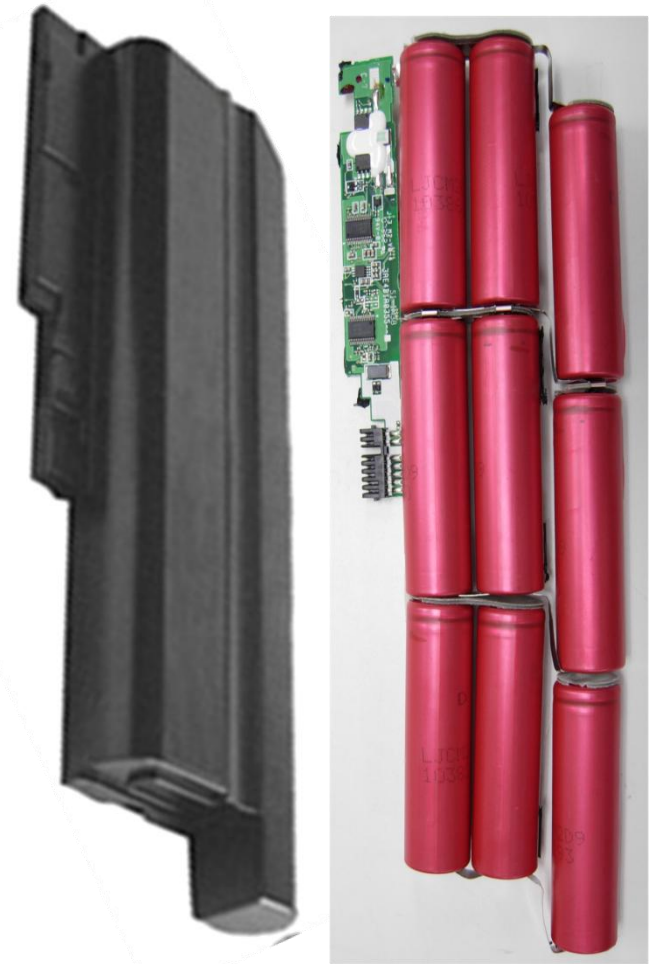
Lenovo Li-ion Battery (ISS) Matrix Design
