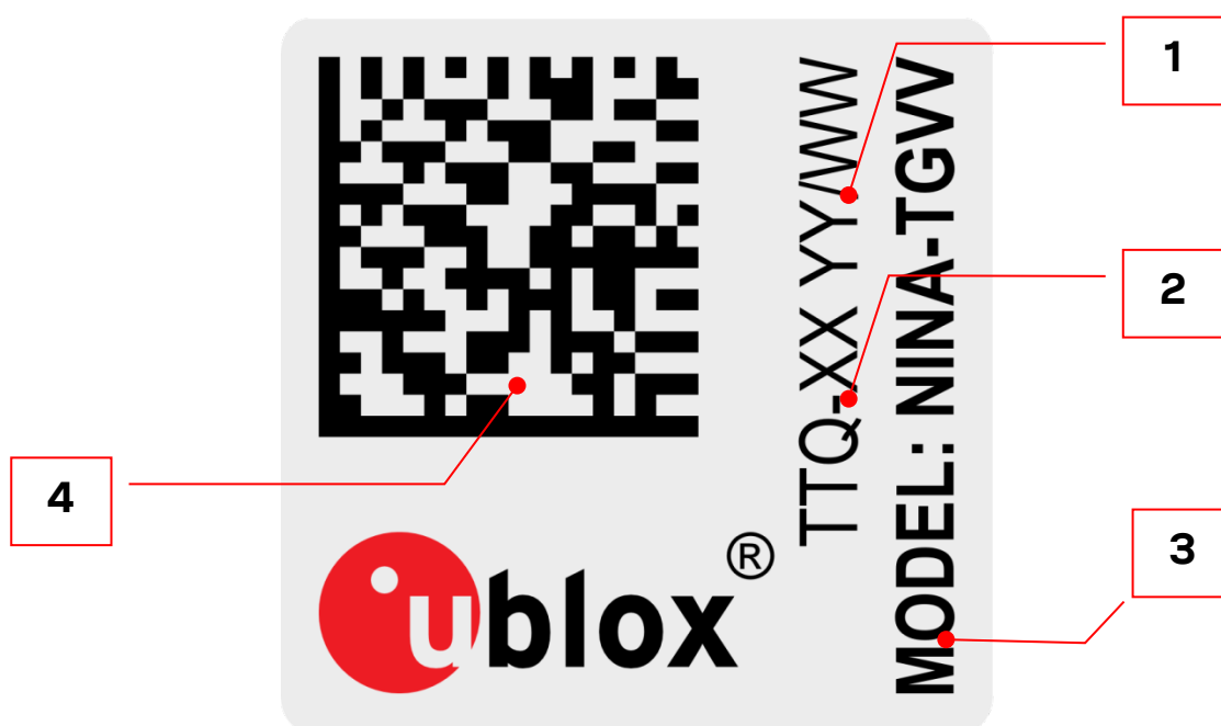
Figure 14: Location of product type number on the NINA-B3 series module label
