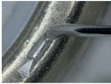
Wire bond on the negative terminal of a cylindrical cell
