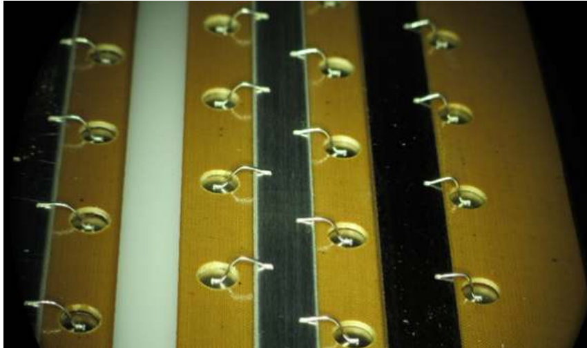
Wire bonded battery pack for Formula SAE Race Car. Photo courtesy of Purdue University Race Team.
