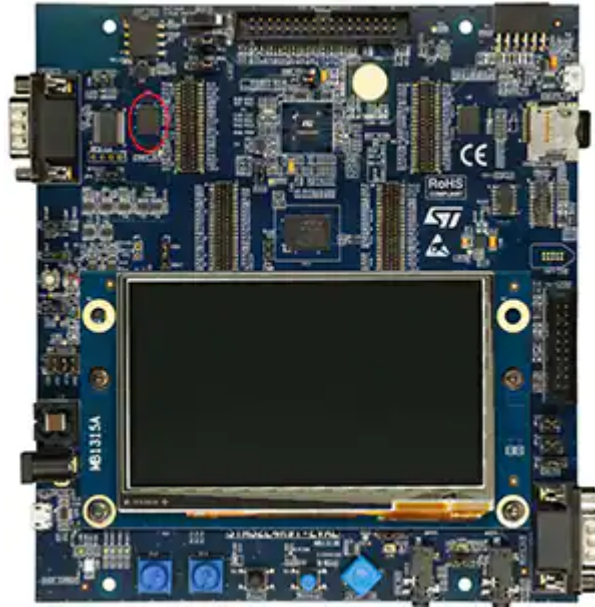
Figure 3: The STMicroelectronics STM32L4R9I-EVAL is used to evaluate the STM32L4R9 microcontroller. The HyperRAM memory device is circled in red with the device's test points located on the header connector to the right. (Image source: STMicroelectronics)
