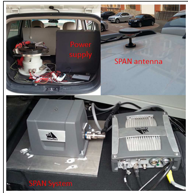
Figure 6. Equipment set-up on the test vehicle.
