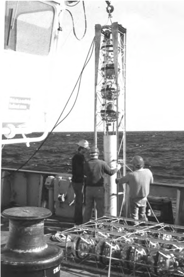
5) Deep SOFAR float using glass spheres. The uppermost sphere provides buoyancy, the middle two hold batteries and bottom sphere contains electronics. The float is seen in a deployment cradle that was opened hydraulically when the float was below the sea surface.(Photograph John Gould)
